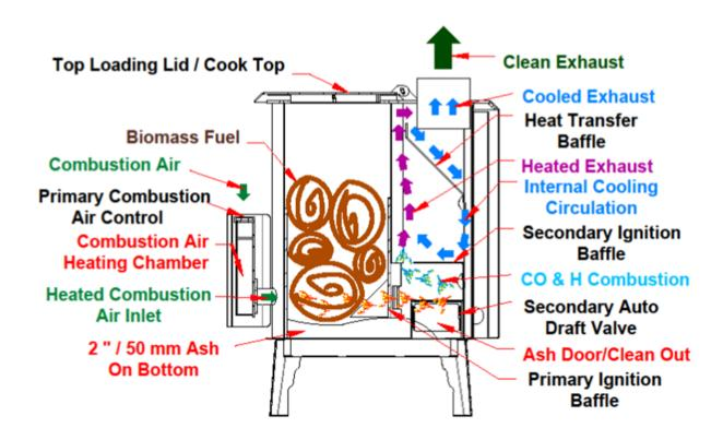
The intake air is admitted through the holes in the crests of the corrugated front wall. This provides a cross draft, which makes the fuel burn only at the bottom of the firebox, or fuel load. As the fuel burns, it's being lowered from above into the burning area. This is how such long burn times are accomplished. The heat output can be regulated from low to high; depending upon the amount of air entering the stove.
