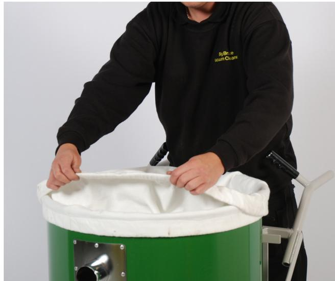
**Fit the Primary Filters inside the top of the drum.**
