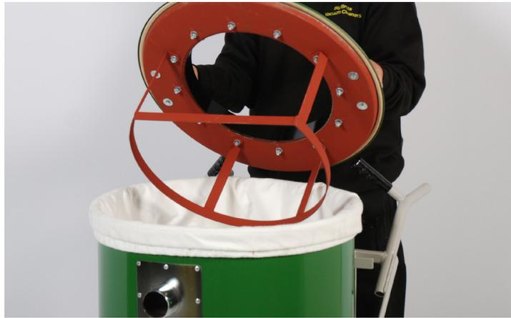
**Fit the lid with the flat bar in the inner frame facing the front of the drum**
