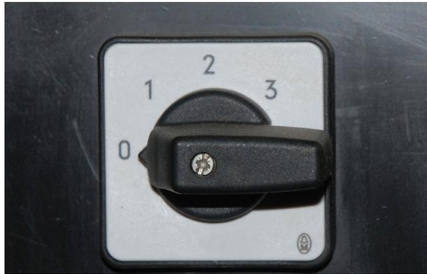
4-position switch for turning on the motors
