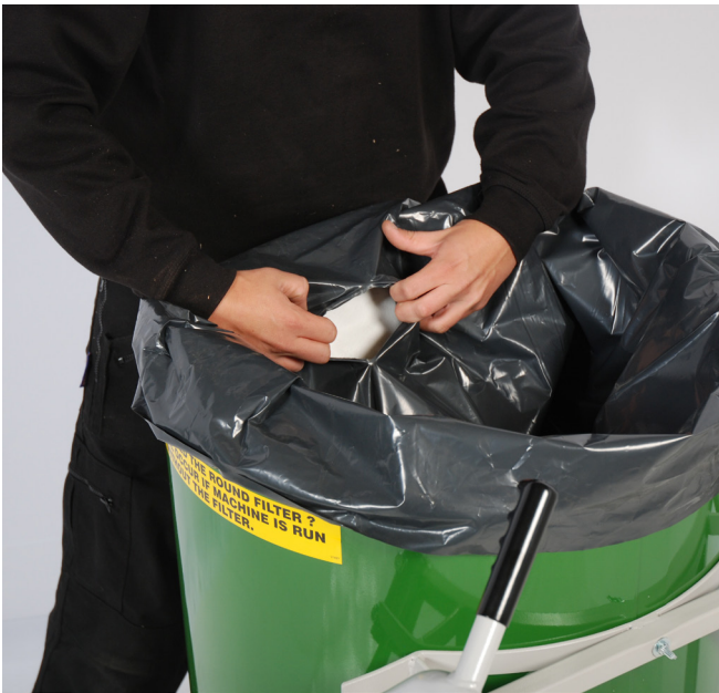
Feel for the inlet spigot behind the waste bag and tear a small hole in the bag
