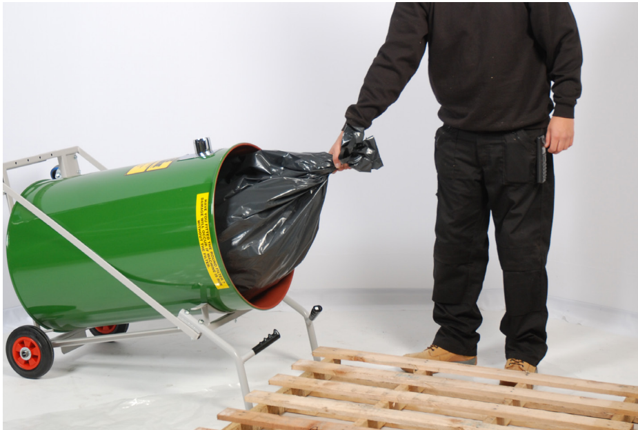
Tie the top of the waste bag off and pull out of the drum.
