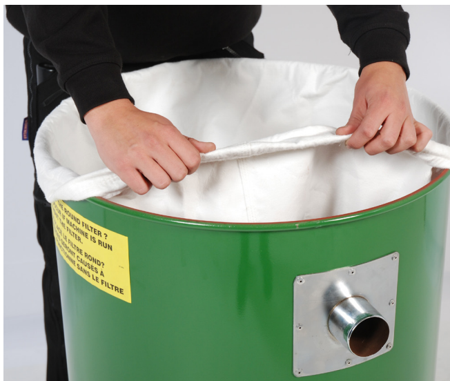
Fit the Primary Filter inside the top of the drum.
