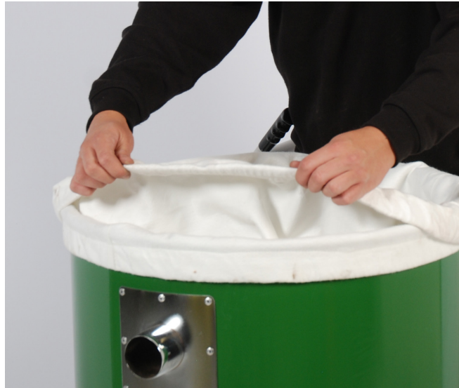
Fit the Primary Filters inside the top of the Leapfrog Drum.
