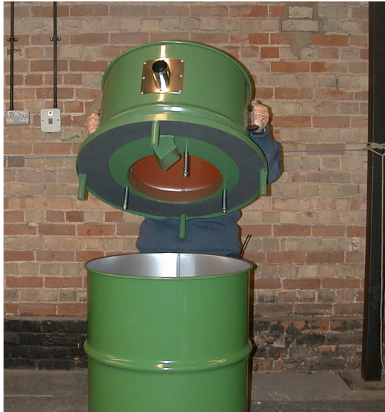
Place the Leapfrog Body onto your collection drum
