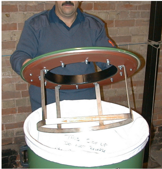
Place the Lid inside the Primary Filters
