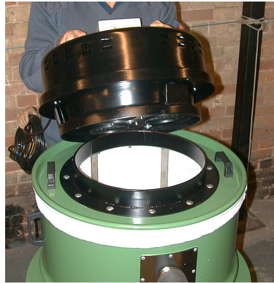
Place the Power Unit on top of the Lid
