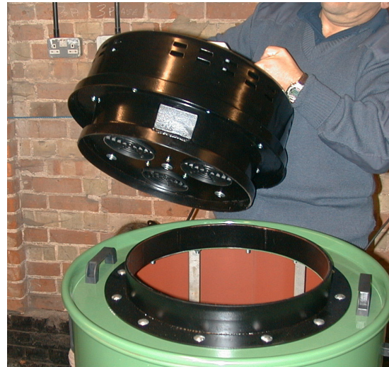
Place the Power Unit on the Lid
